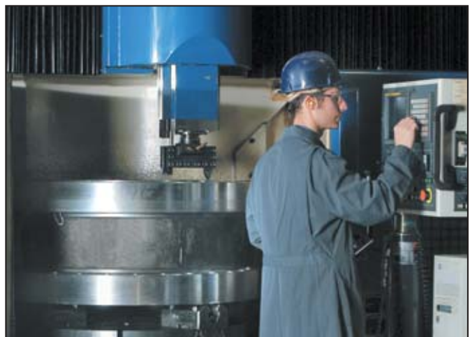
A vertical work station with live spindle, working on a 36" Class 300 Double Flanged Type PF valve body, allows for turning, milling, drilling and tapping operations as applicable in one set-up.
